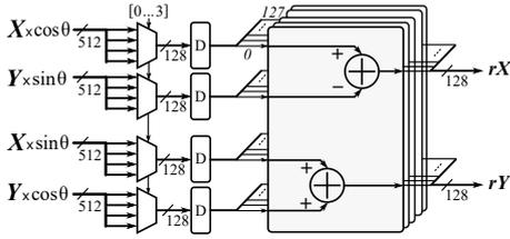
Fig. 6: 4-folded Circuitry of *AddSubVec* block in the *Rotator* unit.
