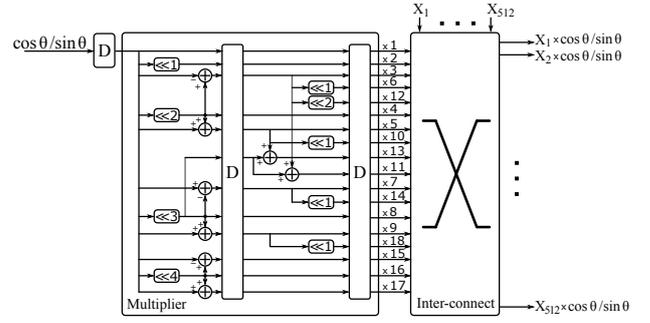
Fig. 5: Circuitry of *Mult Block* in the *Rotator* unit.
