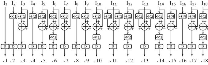
Fig. 4: Implementation of *Mult Block* in the *Centroid* unit.
