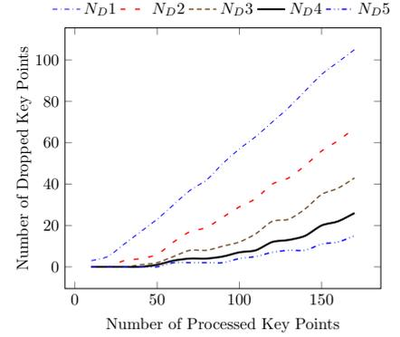
Fig. 10: Dropping rate for different number of replications of the descriptor generator components.
