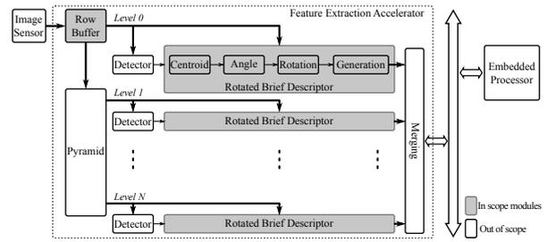
Fig. 1: Architecture of a typical multilevel Feature Extraction Accelerator.
