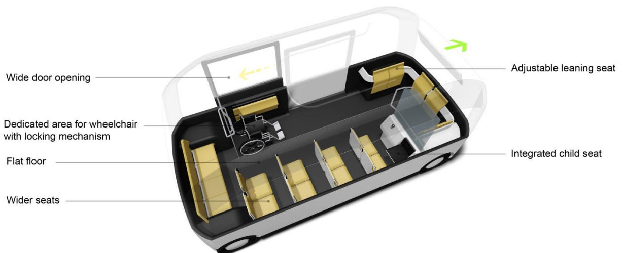
Fig. 4. Interior design of the DART module and main features according to Universal Design principles
