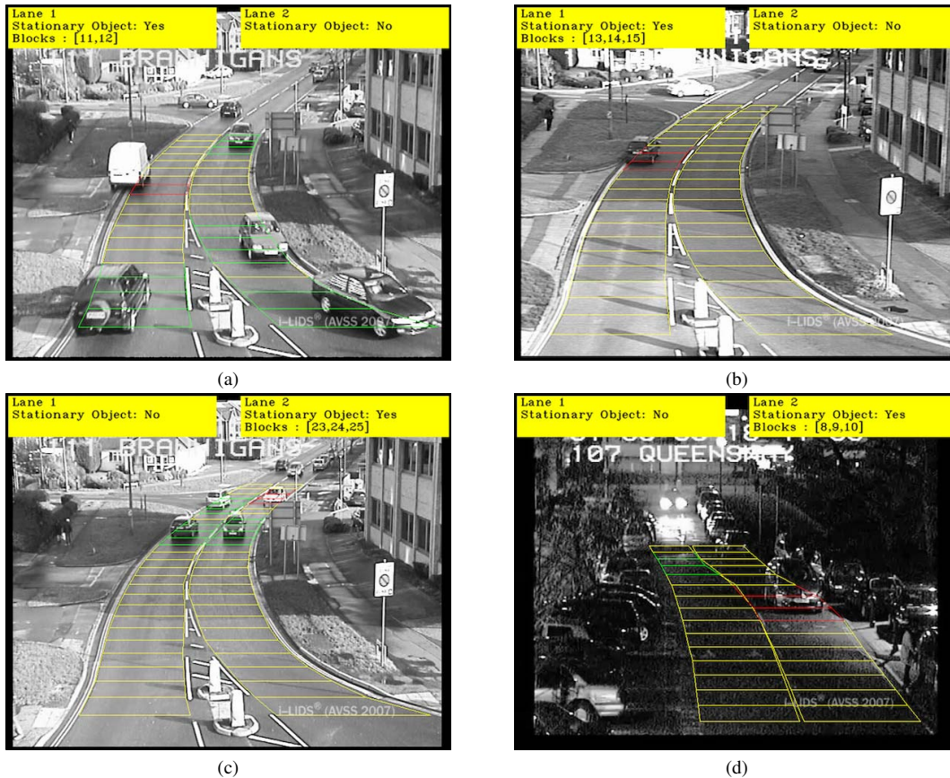
Fig. 3: Detection of Stationary Foreground Object for (a) iLids-Easy (b) iLids-Medium (c) iLids-Hard (d) iLids-Night
