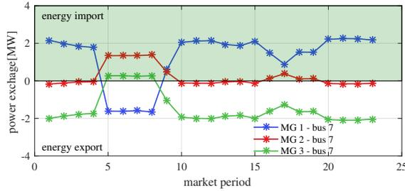
Fig. 5. Import and export power for MG 1-3 on the coupled bus 7 (energy import: positive values; energy export: negative values).
