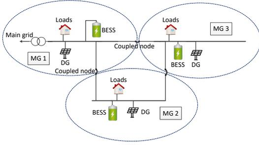
Fig. 1. Multiple MGs with distributed generations and energy storage.
