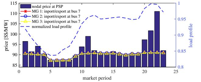
Fig. 3. Nodal price/load profile sample of Singapore's grid are taken from EMCS [14] Singapore on 02/09/2018. The exchange price are recovered from ADMM for the coupled bus for MGs 1-3.
