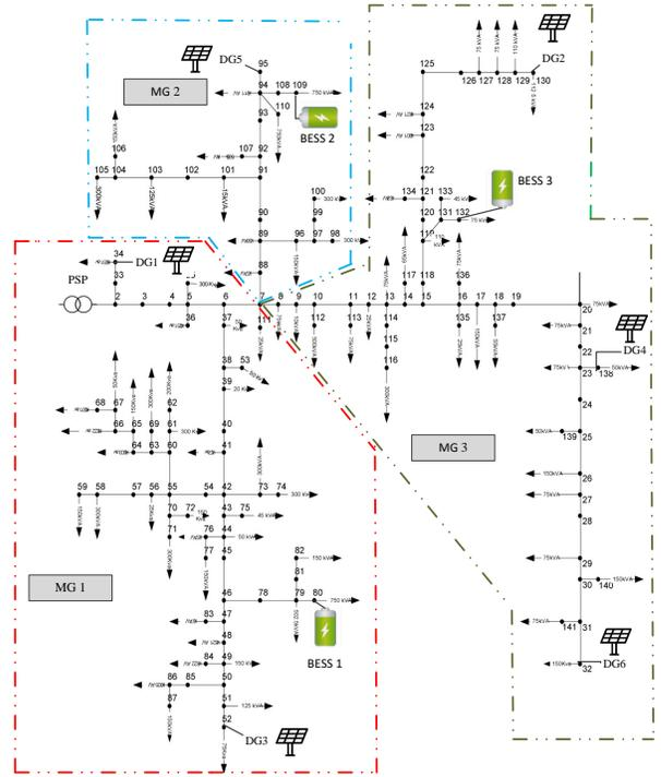
Fig. 2. 144-bus network partitioned into 3 MGs with 6 DGs and 3 BESSs.
