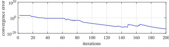
Fig. 6. Convergence error (the sum of primal residual:  $\sum_{i=1}^s r_i^2$ ).
