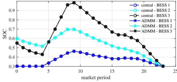
Fig. 4. SOC results: comparison of ADMM to centralized solution.
