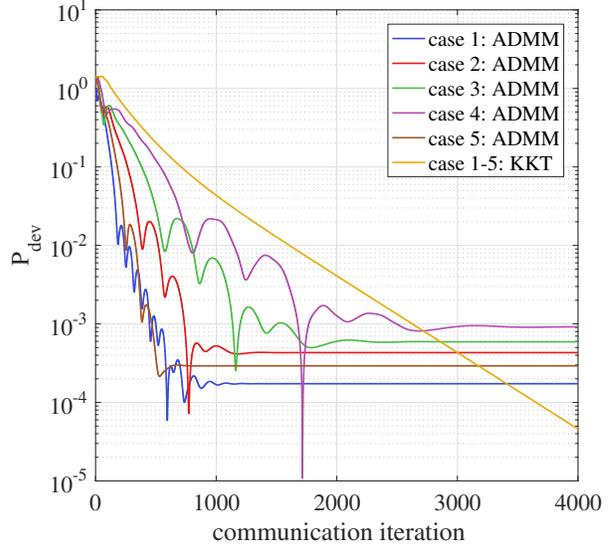
Fig. 4. Standard deviation to optimal power generation
