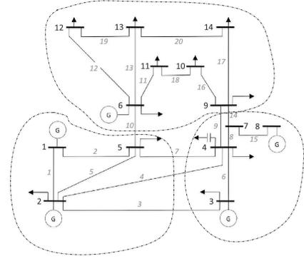
Fig. 2. IEEE 14 bus test case with three clusters
