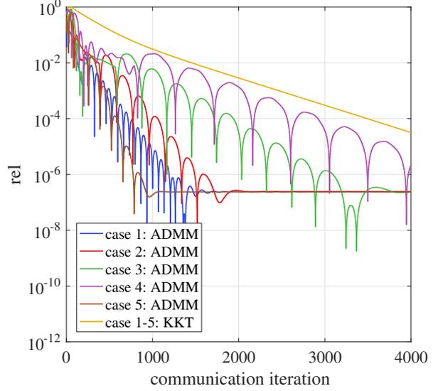
Fig. 3. Deviation to optimal generation cost
