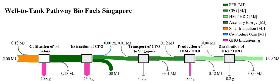
**Figure 6: Energy flow and GHG emissions for hydrogenated renewable jet fuel and diesel in Singapore**
