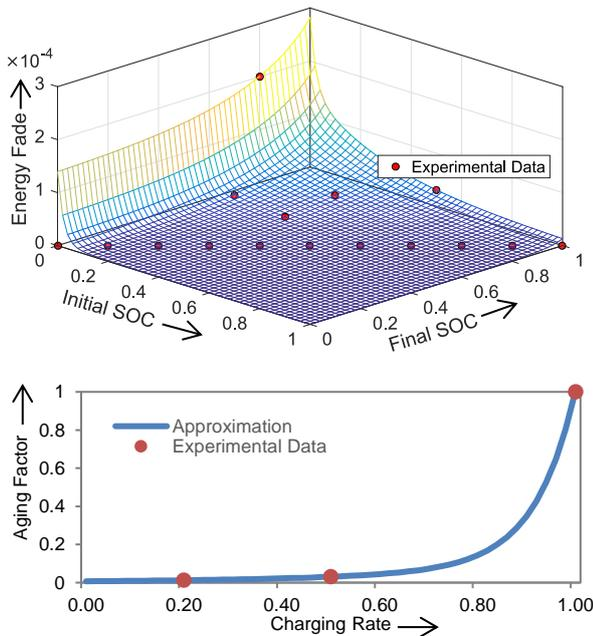
Figure 9. Battery aging parameters: energy fade (top), aging factor (bottom).
