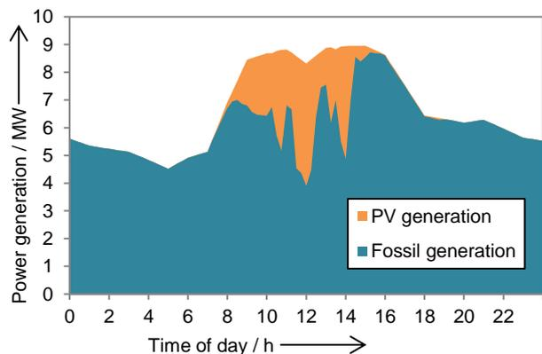
Figure 10. Fossil and PV generation on a day with high fluctuation of PV power output and no EVs.
