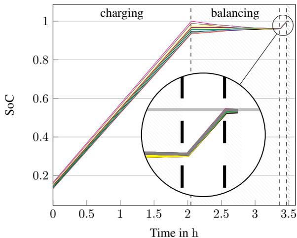
Fig. 3: Conventional charging process. Alternating charging and balancing phases to achieve full charge will extend the time the vehicles is connected to the charging station.
