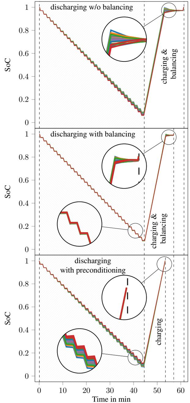
Fig. 7: Development of the cell's SoC during a round trip with 31 stops and subsequent charging phase. **Top:** discharging with subsequent charging and balancing phase. **Center:** discharging with balancing and subsequent charging and balancing phase. **Bottom:** discharging with preconditioning for minimized charging time and subsequent charging phase. No balancing required while charging.
