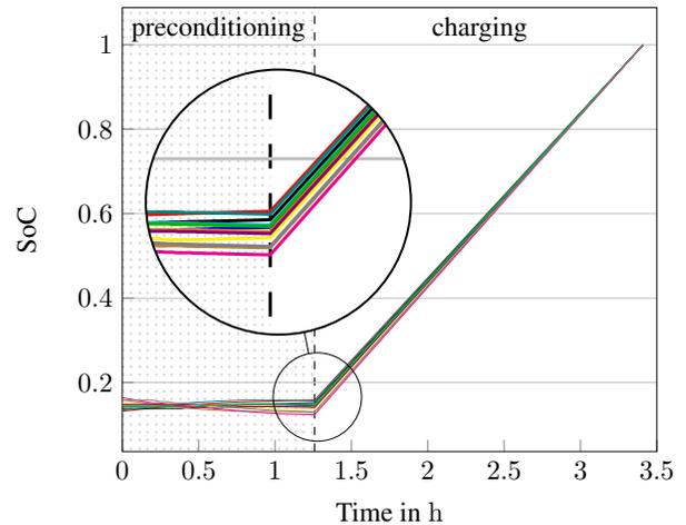
Fig. 6: Preconditioning process. The preconditioning phase (dotted) is followed by only one charging phase resulting in all cells of the battery pack to be fully charged at once.
