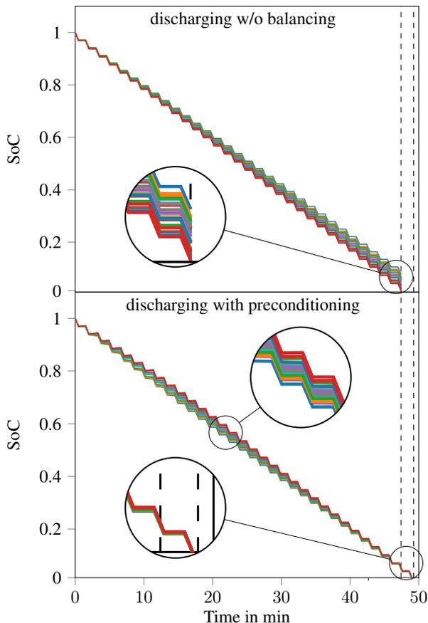
Fig. 8: Development of the cell's SoC during discharging. **Top:** discharging conventionally. **Bottom:** discharging with preconditioning for maximized capacity.
