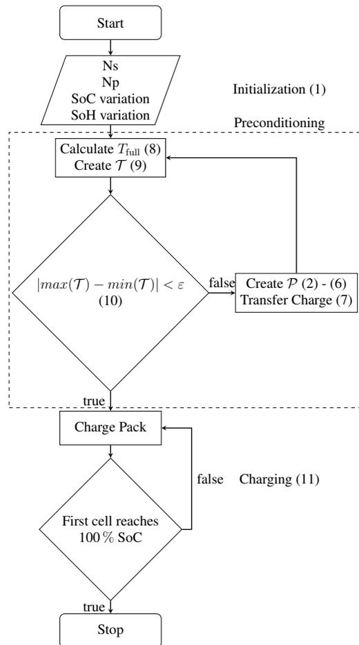
Fig. 4: The preconditioning algorithm highlighting the relevant steps in a charge cycle with preconditioning.
